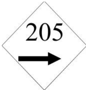
Figure 3: Detour Sign – Rte 205 diverted right
